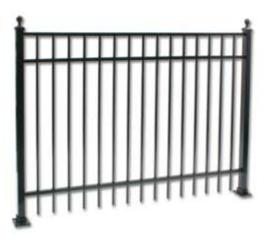
Rails: 1"x.055" thick Pickets: 5/8"sq x.050" thick Line/End/Corner Posts: 2"sq x .060" thick Gate Posts: 2"sq x .125" thick Picket Spacing: 3 13/16" Post Spacing: 72 1/2" on center Height: 48" & 60" Range of angular adjustability (rackability): 30" over a 6' section
